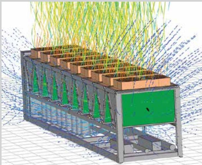
CFD analysis was used to determine the optimum fan and heat exchanger size and the best distribution and total airflow through the V - block to minimise power consumption
